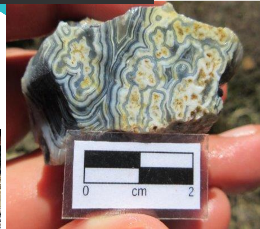
Above: Aloe Eumpeuk sample showing colloform banding fine sulphides epithermal quartz
